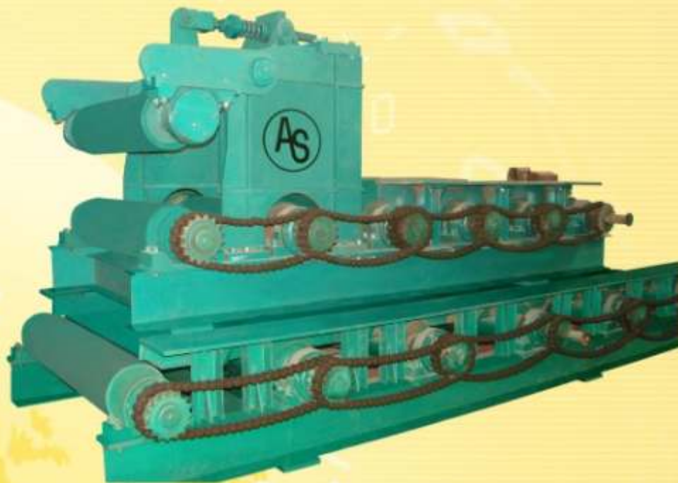
Furnace Discharge Table cum Pinch Roll
